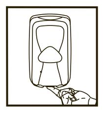
**1.** Open dispenser by pushing release on bottom of dispenser and pull down on front cover.
