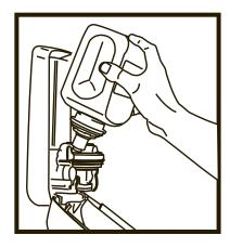
**3.** Insert refill at slight angle into dispenser so nozzle is inside lock release.
