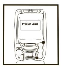
**4.** Fully insert refill down into lock release until refill clicks into place.
